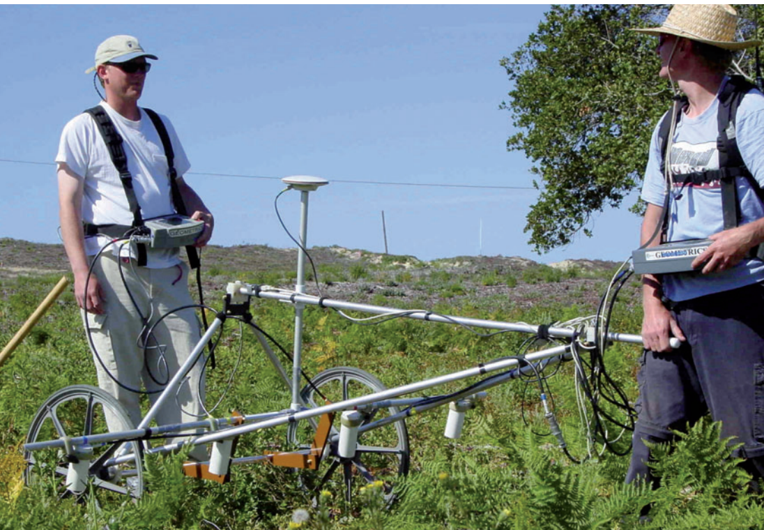
Cart with 3 sensors mounted
