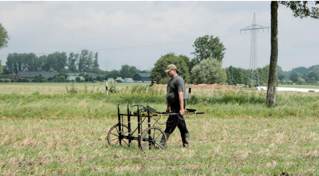
The FEREX 4.032 DLG (datalogger) multi-sensor detection with wheel set.
