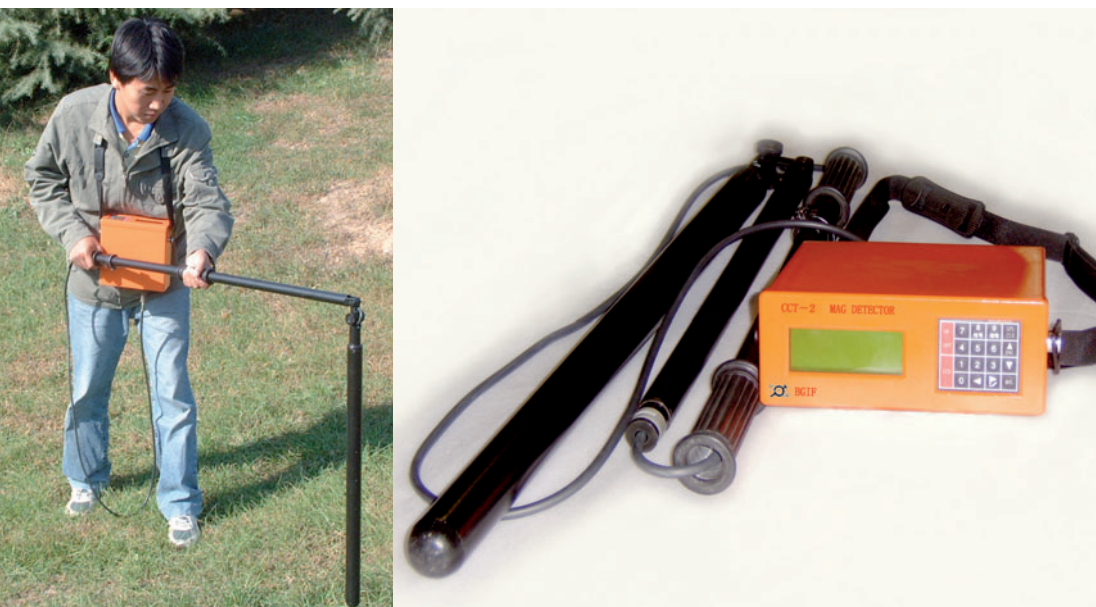
The CCT-2 Magnetic Detector in service
