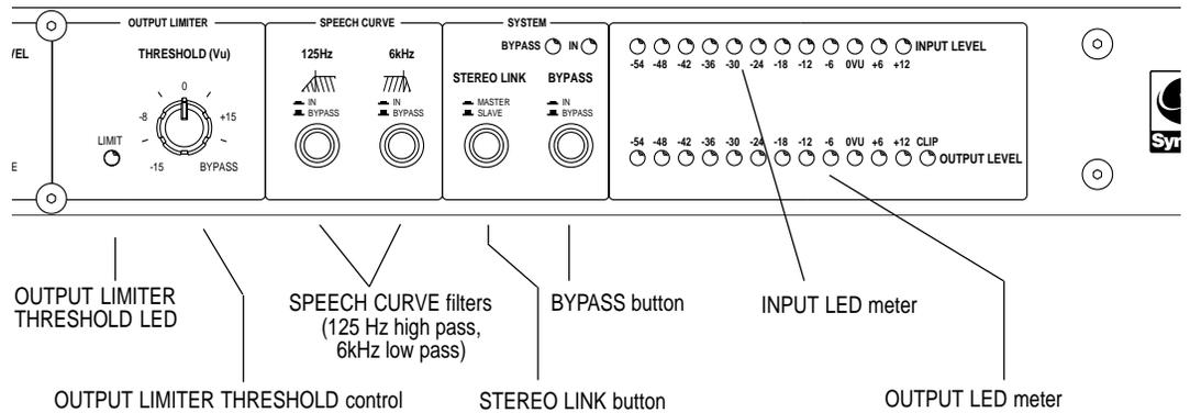
**OUTPUT LIMITER THRESHOLD LED** - Indicates peak limiting activity.
