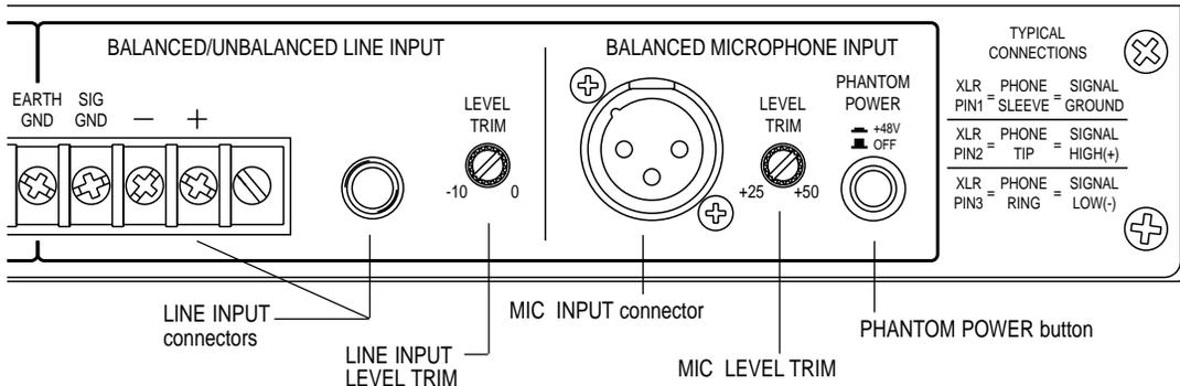
**LINE INPUT** - These connectors are electronically balanced, line level, bridging inputs. The 1/4" connector tip is high, ring is low, and sleeve is ground. The screw terminal input is wired in parallel to the 1/4" connector.
