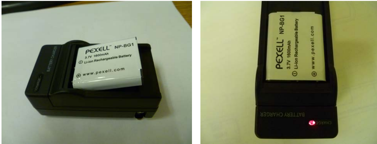
Figure 1-12: Placing Extended Marker Batteries into Charger
