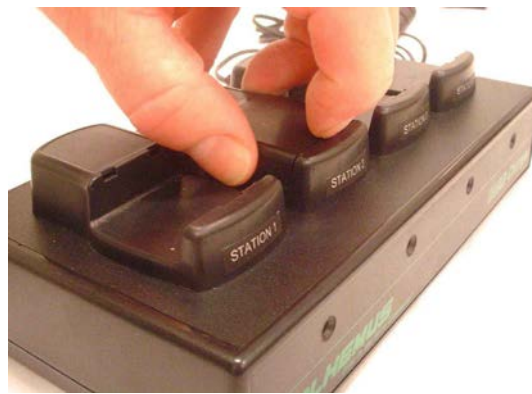
Figure 1-21: Standard Marker: Preparing to remove the battery
