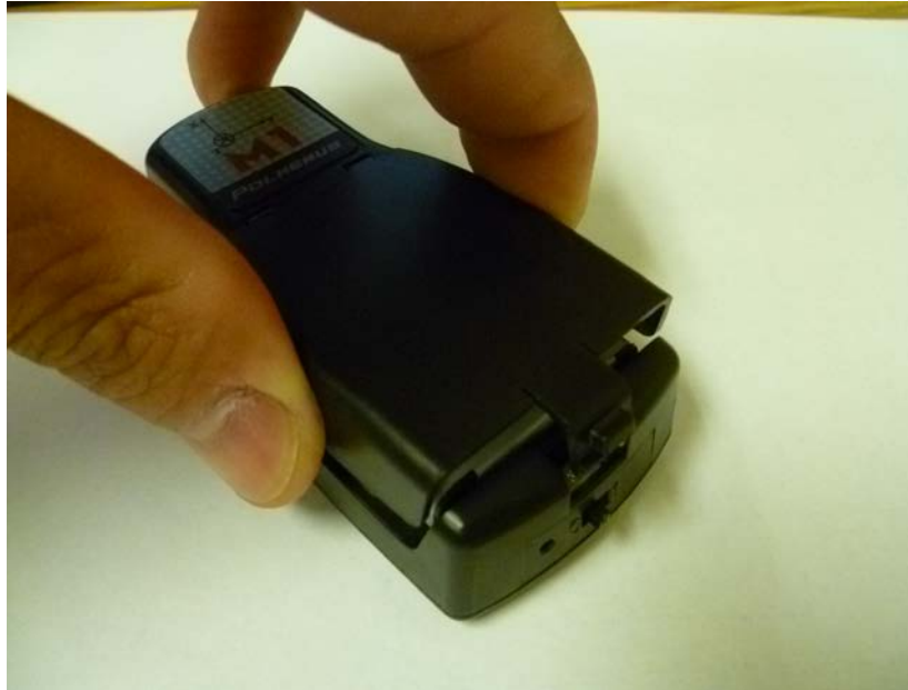
Figure 1-14: Extended Marker Battery Insertion
