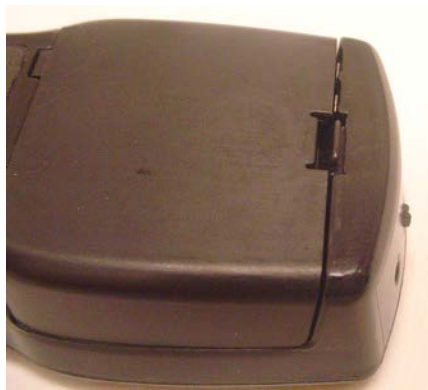
Figure 1-26: Proper seating of spring clip
