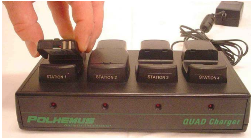
Figure 1-18: Standard Marker: Placing Batteries into Charger
