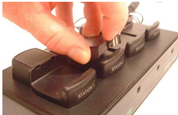
Figure 1-22: Standard Marker: Lifting the battery
