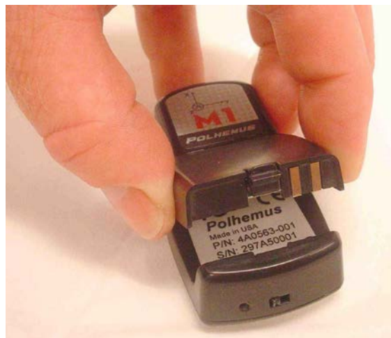
Figure 1-24: Standard marker battery insertion
