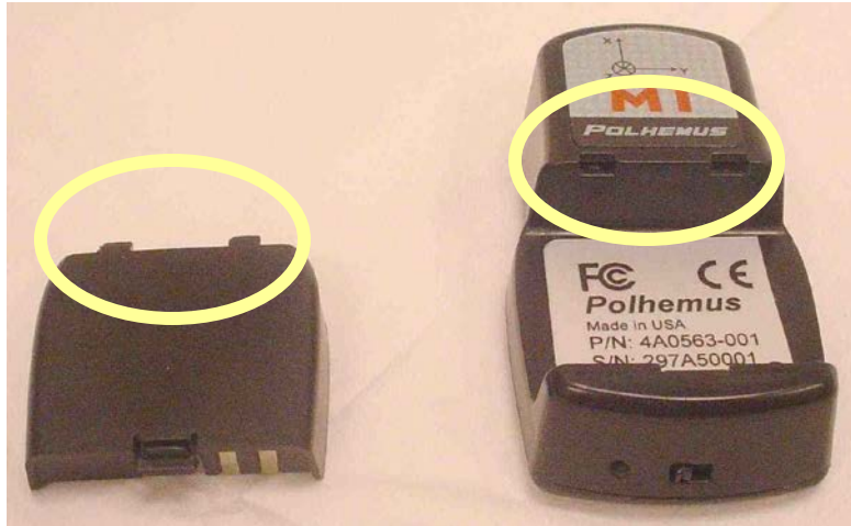
Figure 1-23: Standard marker battery tab orientation
