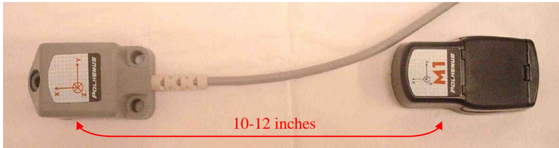
Figure 1-5: Receptor/Marker Test Setup
