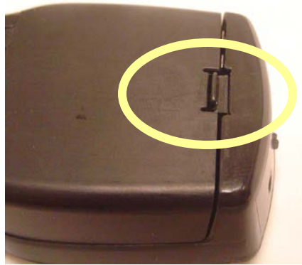
Figure 1-25: Spring clip improperly seated
