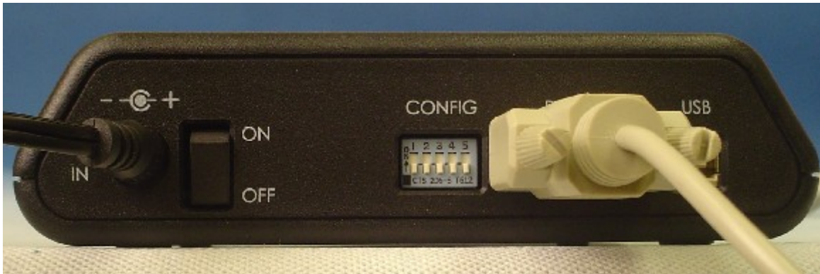
Figure 1-9: RS-232 Cable Connection
