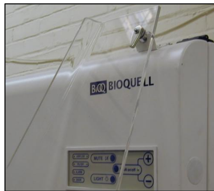
Figure 3: Window secured open with lock located in top bracket
