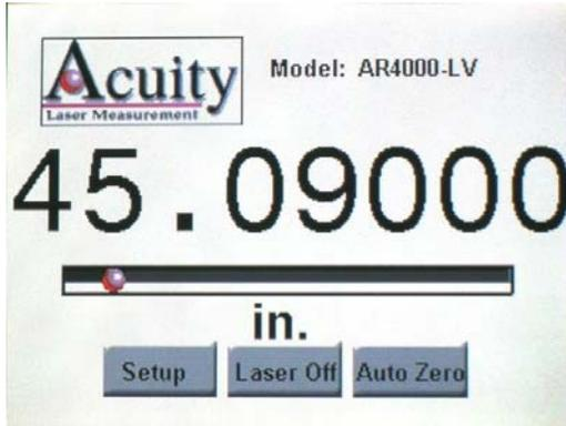
The Main Display Screen with measured value within limits displayed in black
