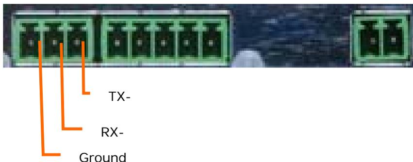
**Figure 2. Function of individual RS232 terminal blocks**
