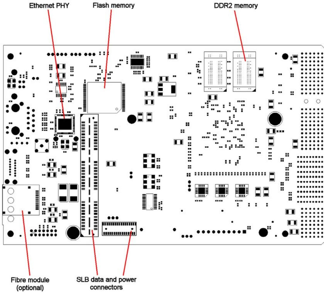
Figure 10 Bottom-side of SMT700 Carrier
