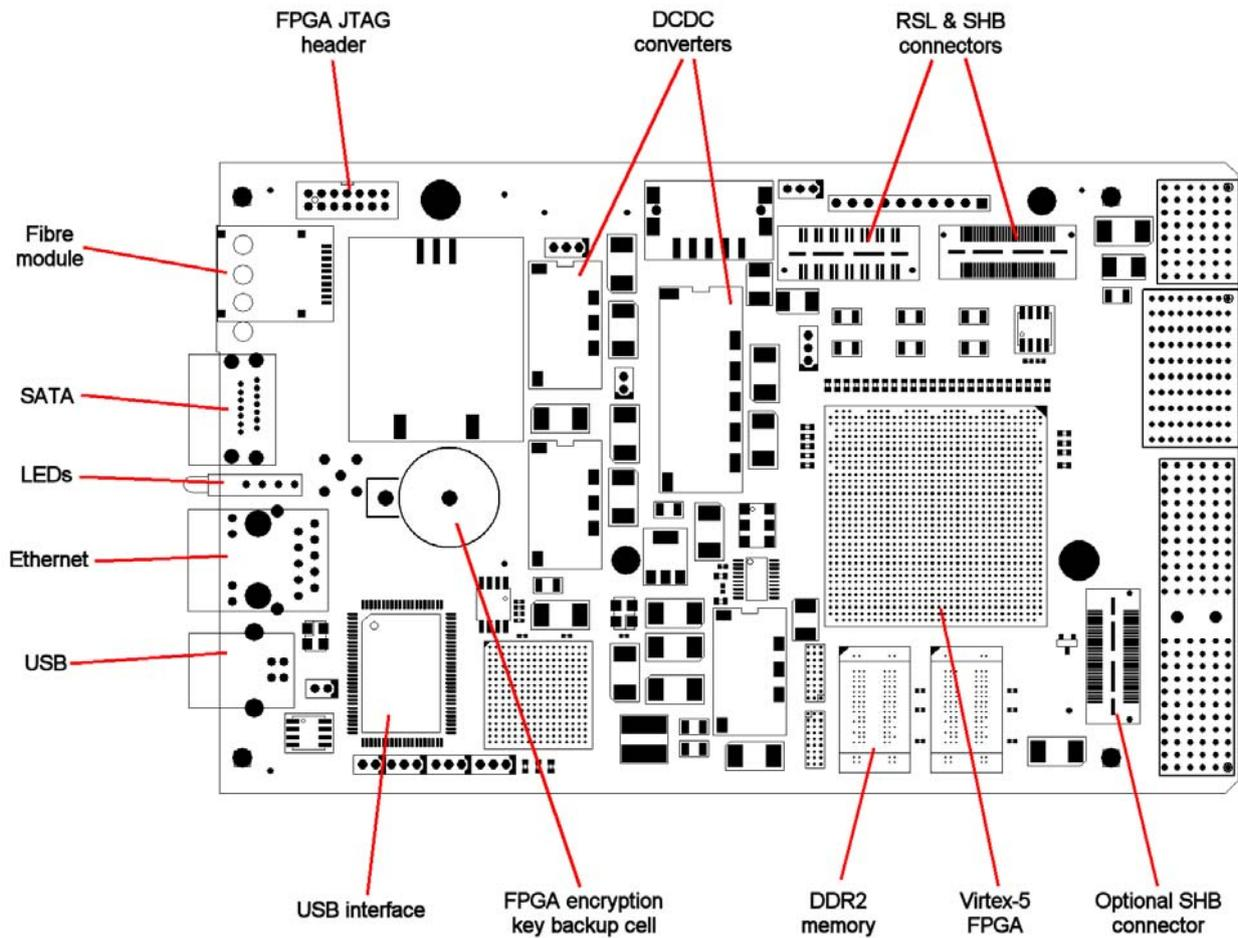
Figure 9 Top-sid of SMT700 Carrier
