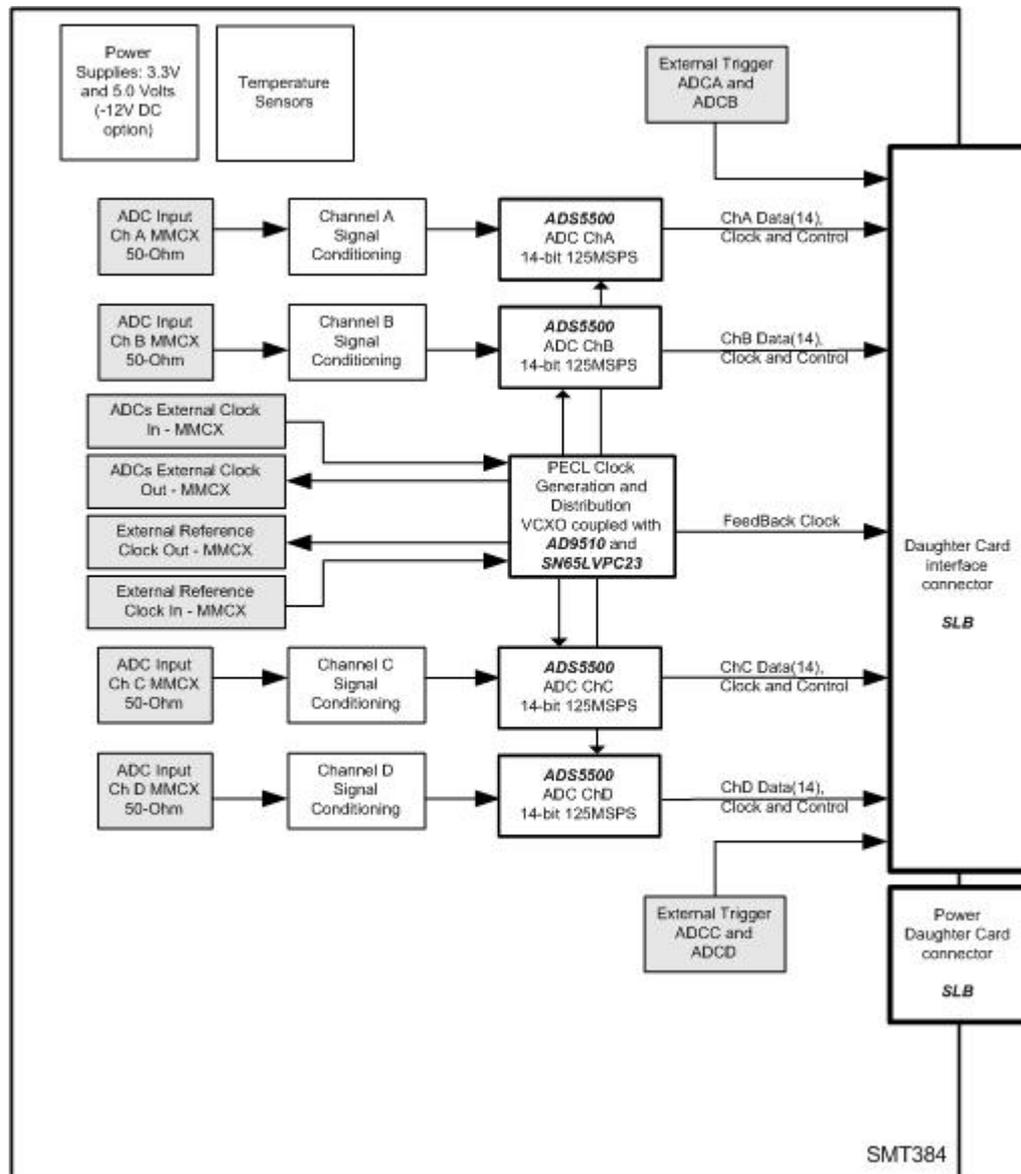
Figure 2 SMT384 Block Diagram
