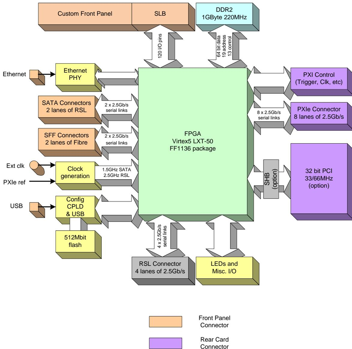
Figure 1: SMT700 Block Diagram
