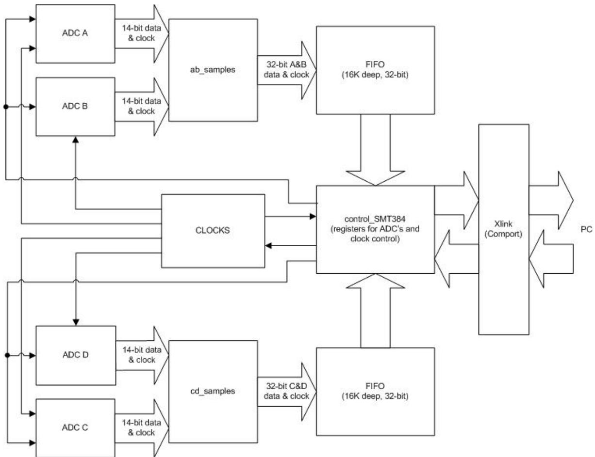
Figure 5 ADC Data Flow
