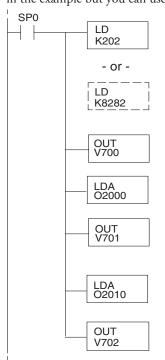
Loads a constant that specifies the number of channels to scan and the data format. The upper byte selects the input data format (i.e. 0=BCD, 8=Binary) and the number of input channels (set to either 1 or 2 for the F0-2AD2DA-2). The lower byte selects the output data format (i.e. 0=BCD, 8=Binary) and the number of output channels (set to either 1 or 2).
