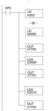
Load a constant that specifies the number of channels to scan and the data format. The upper byte selects the input data format (i.e. 0=BCD, 8=Binary) and the number of input channels (set to either 1 or 2 for the F0-2AD2DA-2). The lower byte selects the output data format (i.e. 0=BCD, 8=Binary) and the number of output channels (set to either 1 or 2).
