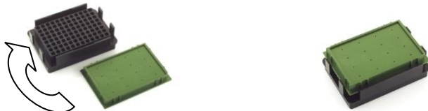
Figure 20 - The Roche 1536 adapter (4ti-0616) should be placed inside the adapter for 96well PCR plates (4ti-0625). This adapter is required for Roche 1536well plates.
