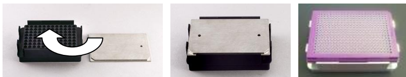
Figure 17 - The standard plate carrier (4ti-0615) can be placed inside the adapter for 96well PCR plates (4ti-0625). This is recommended for skirted shallow well plates, such as 384well PCR plates
