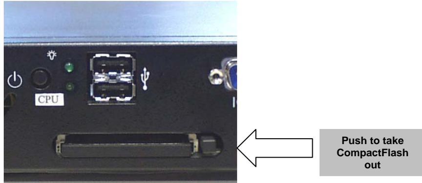
Figure 7. CompactFlash Adapter
