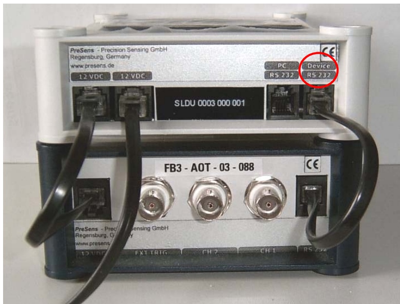
Picture 1: Connection between control panel and oxygen instrument
