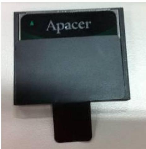
**Step 3** Insert the CFast card to the CFast card slot, then finding the CFast cover and screw it.
