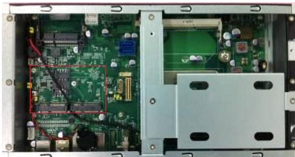
**Step 2** Insert the wireless LAN card to the slot. Push it down firmly until it is clipped by the slot.
