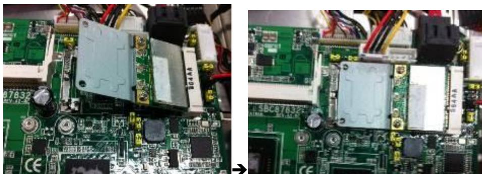
Step 3 Find the Antenna cable and connect it on wireless LAN card.
