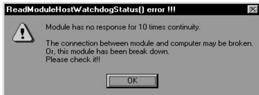
Figure 3-16. Module Status - Communication line is broken.
