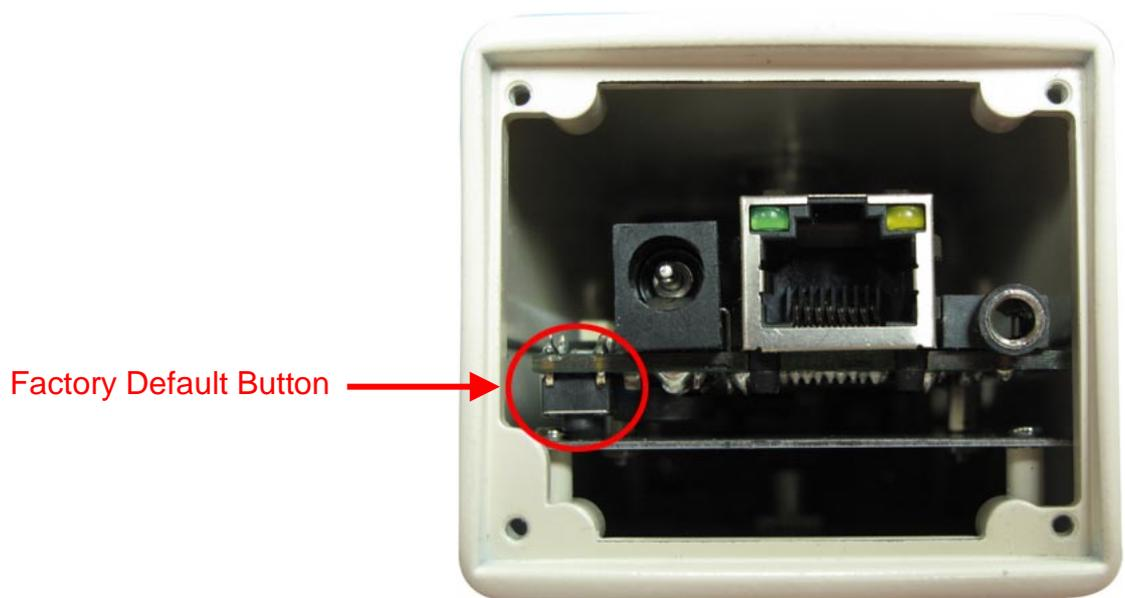
4. Power on the device. Don't release the button during the system booting.
