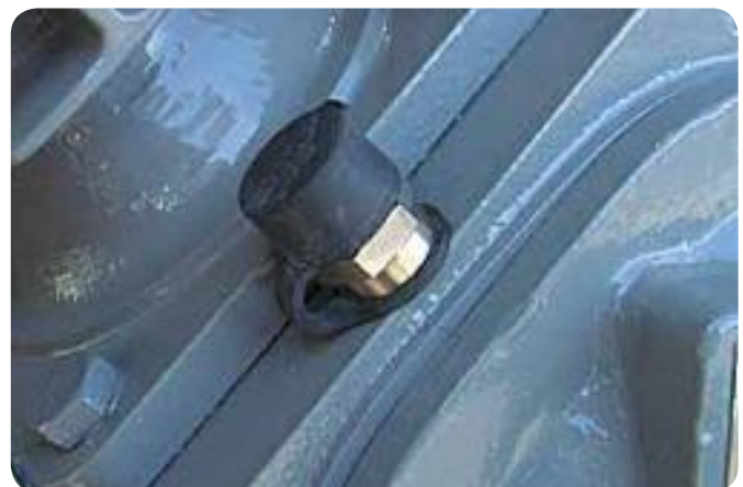
Installed SKF MARLIN QuickConnect (MQC) stud with protective cap
