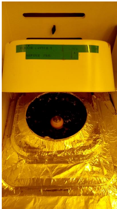
Fig.5 Spinner Chuck, Spindle Motor, Coating Chamber with Lid and Heavy Duty Aluminum Foil covering to maintain a clean around the coater
