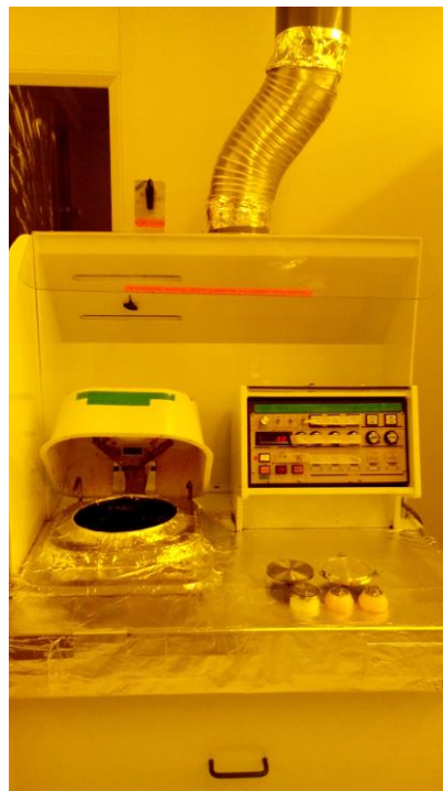
Fig.3 Controller Front Panel and Spin Coating Chamber with Lid
