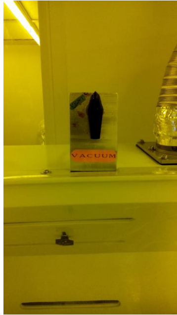
Fig.6 Vacuum Ball Valve for applying vacuum to the chuck
