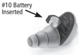
**Note:** The door will not close if the battery is not inserted correctly.
