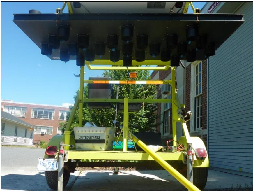
2. Open the black interface panel case (the one standing vertical) and pull out the two cables – the black camera cable, and the yellow interface panel power cord, through the hole at the bottom of the case.
