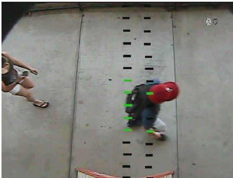
Initially, when a detector is not covered by a pedestrian or vehicle, it has an "off" status. Video streamed from the camera to the PC shows these "off" detectors in black. When a pixel in the
