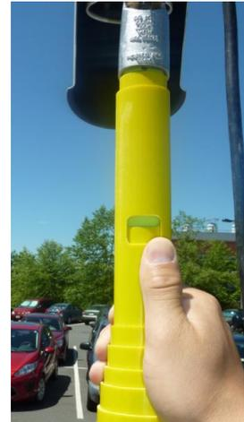
6. Disconnect the camera cable, unscrew the camera from the mast and store it in the storage case.
