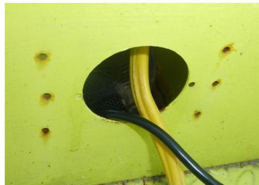
13. Use the Ethernet cable to connect the interface panel and the laptop. One end of the cable is connected to the Ethernet port of the Autoscope interface panel, while the other end is connected to the Ethernet port of the laptop. Pass the cable through the bottom hole of the interface case and through the side hole in the laptop case.
