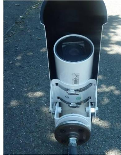
6. Attach the camera cable from the interface panel to the camera as shown in the picture. Markings on the cable plug and the camera socket can be matched to fit the plug correctly. Flip down the latch on the cable, to lock the cable and the camera together.
