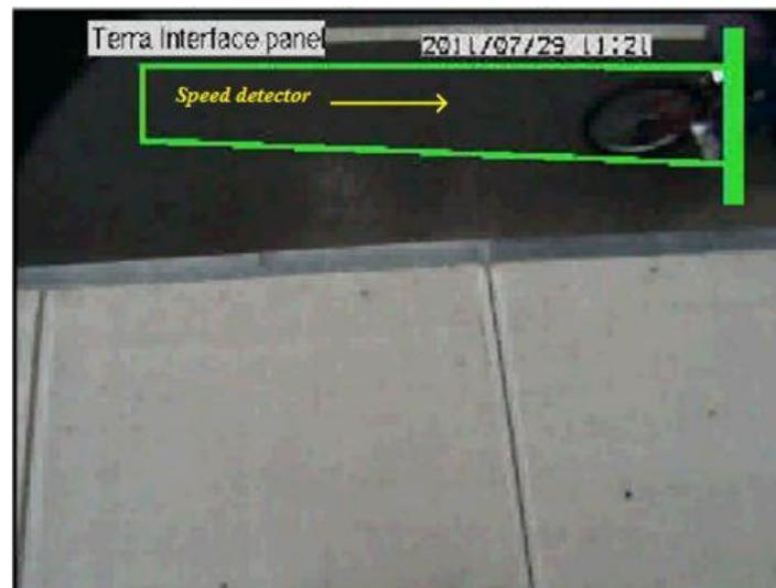
To address this difference, the Solo Terra camera was used in a slightly different way to detect bicyclists versus pedestrians. To detect bicyclists, a speed detector was used. In this case, it is assumed that bicyclists will travel in a single direction in a lane which adjacent to a sidewalk, as shown in Figure 2.9. Speed detectors, when configured for use with the Solo Terra, measure the speed and length of the vehicle passing through it.
