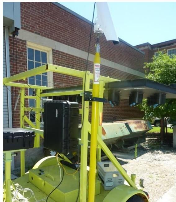
9. Once the mast is secured, draw out the second layer of the mast upwards to the point it is locked with the red button. The first layer is not chosen to make sure that the pole does not sway with wind once the mast is drawn out at a higher level. Using the second layer improves the thickness of the mast, and thus its stability.
