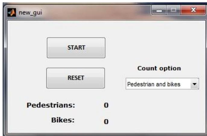
2. The **START** button is used to start the counting process, when the software is started in the beginning. Once the **START** button is pressed, the software continuously keeps counting, and displays the pedestrian and bike count value in real time. The option to stop counting is not available - though the count can be reset to zero at any time using the **RESET** button.
