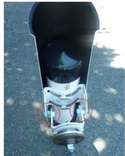
5. Remove the protective lens cover from the camera.
