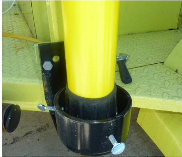
8. Secure the higher end of the mast by fixing the bracket around it. While affixing the bracket tight, make sure that the camera is facing the road, perpendicular to the edge of the trailer.
