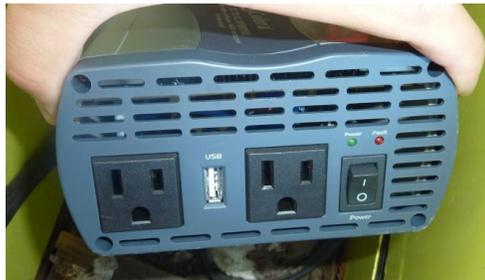
3. Disconnect the inverter from the battery. The inverter can be placed either in the separate storage case or can be left in the battery cabin.
