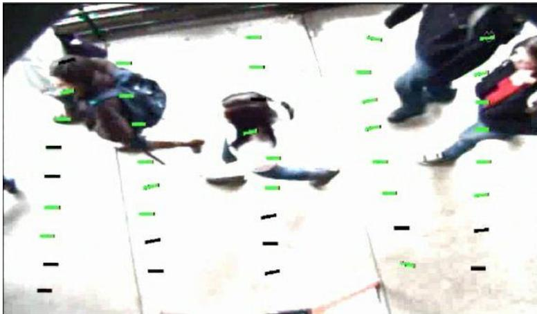
Since the Solo Terra increments the pedestrian count based on changes in pixel values, an approach is needed that validates the count as it is determined.
