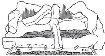
**Figure 45 - Correct Front Burner Flame Pattern**
