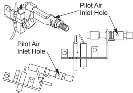
**Figure 48 - Pilot Inlet Air Hole (Your pilot assembly may vary from pilots shown)**
