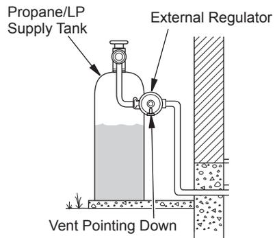
**Figure 20 - External Regulator with Vent Pointing Down**
