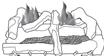
**Figure 46 - Incorrect Front Burner Flame Pattern**
