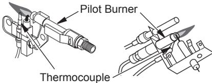
**Figure 43 - Correct Pilot Flame Pattern**
