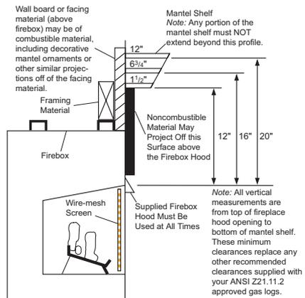
**Figure 6 - Minimum Mantel Clearances for Built-In Installation**
