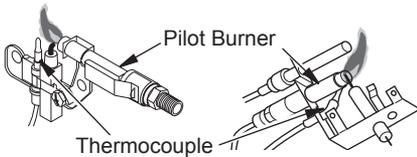
**Figure 44 - Incorrect Pilot Flame Pattern**
