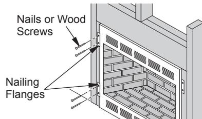
**Figure 8 - Attaching Firebox to Wall Studs**
