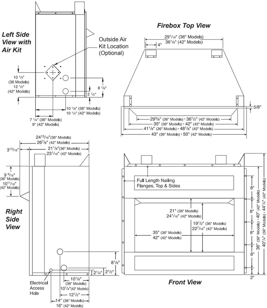
Figure 2 - Firebox Dimensions (36" and 42" Models)
