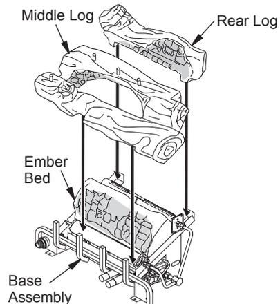
Figure 32- Installing Ember Bed, Rear and Middle Logs
