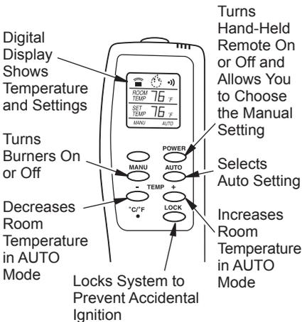
**Figure 42 - Thermostat Hand-Held Remote Control Unit (GHRCTB)**
