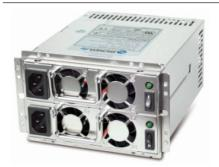
A dual redundant PSU is fitted, input 90-264VAC, 47-63Hz, 600 W with twin AC power inputs on standard IEC fixed plugs. In the event that one power supply fails, the other one takes over the full load without interruption. A defective power supply may be exchanged during operation to ensure high system reliability.
