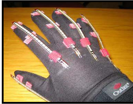
Figure 1.2.3: Music is Possible I Device (Flex Sensors Shown disconnected)
