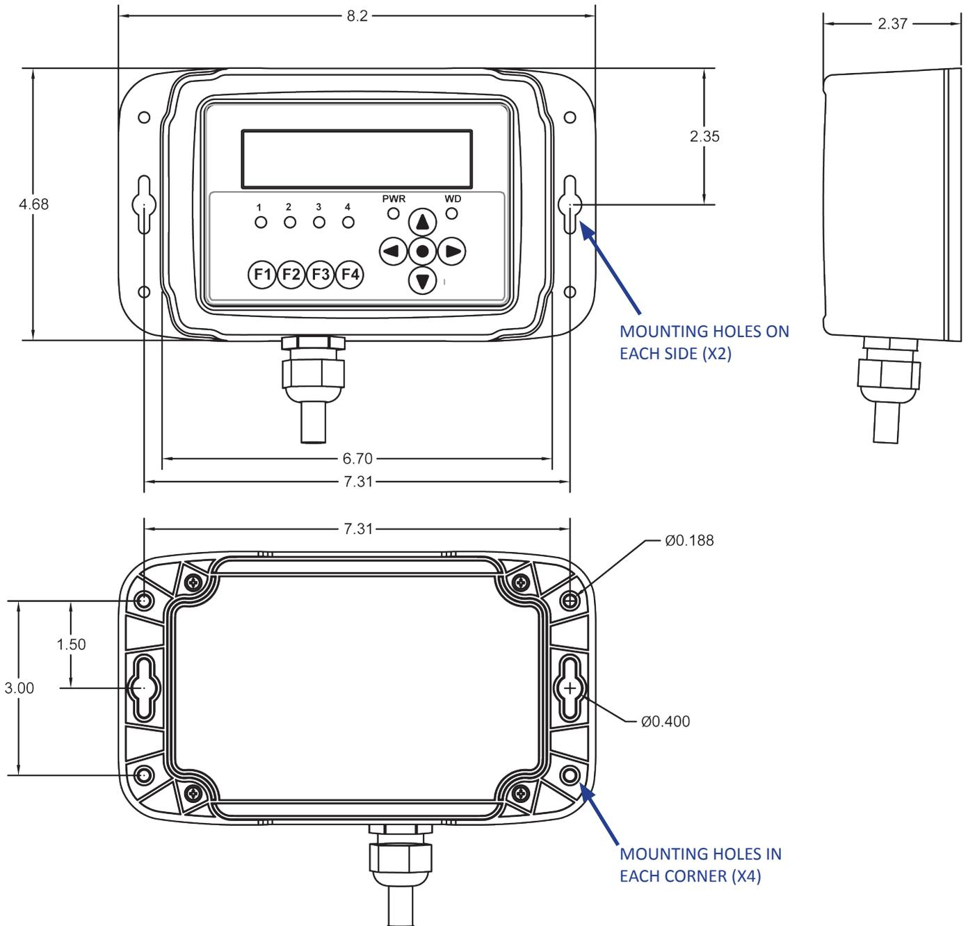
**Figure 9 - Mounting & Dimensions**
