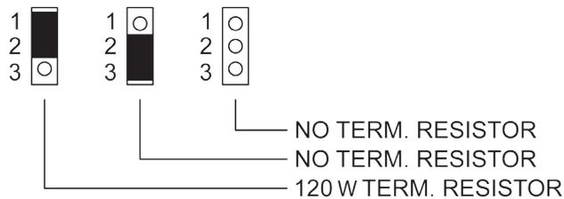
Figure 20 - CAN Port Terminating Resistor Option
