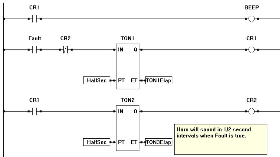
Figure 25 - Programmable Horn - Ladder Diagram
