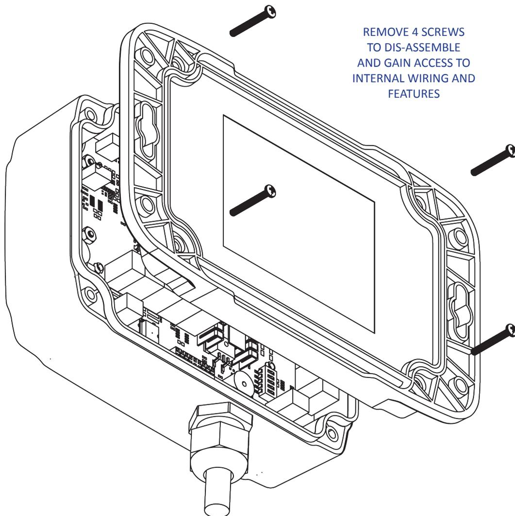
Figure 7 - Assembly / Disassembly
