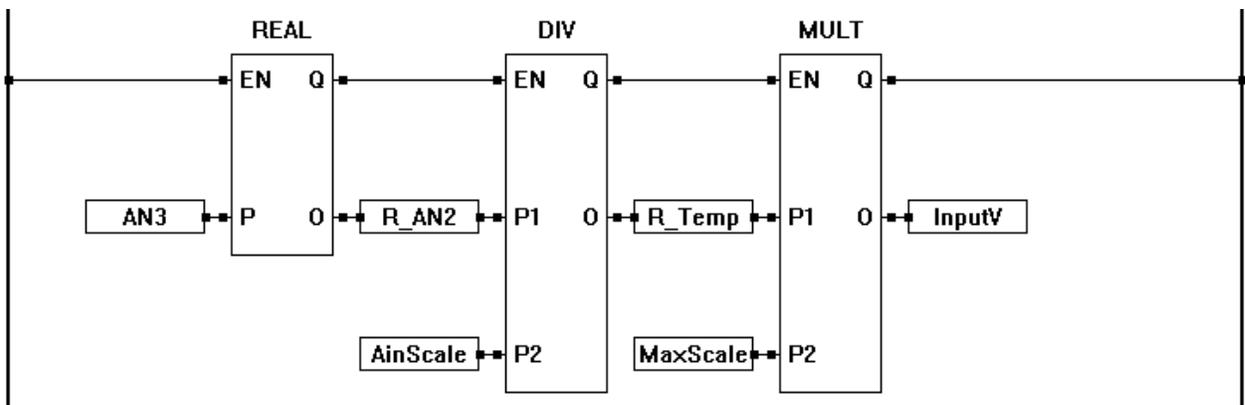
**Figure 11 - Power Monitor Example Ladder Diagram**
