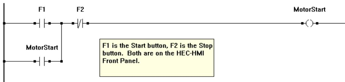
Figure 23 - Programmable Buttons - Ladder Diagram
