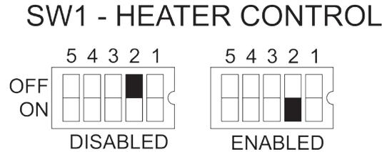
Figure 24 - Field Selectable Heater On/Off Control
