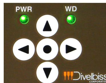
The four remaining buttons are placed to serve as general use buttons. Each button may be programmed and used for any purpose in the ladder diagram project. These buttons are used in the ladder diagram as digital inputs. Contacts (boolean variables) for each button are automatically created when the HEC-HMI model is selected in the Project Settings. These variables are F1 (F1), F2 (F2), F3 (F3) and F4 (F4).
