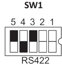
Figure 15 - COM1 RS422 Port Connections
