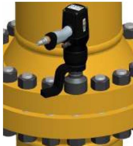
Figure 21 - REACTION ARM AGAINST NEARBY FASTENER
