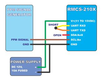
To enable the PPM signal input to the RMCS-220x the UART TXD and UART RXD lines of the RMCS-220x must be shorted together. Remember to power – off and power – on RMCS-220x after shorting RXD and TXD.
