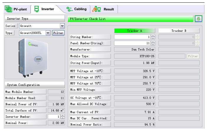
• Cabling: Provide advises and supports for the cabling of the systems. ShineDesign will automatically adjust the specifications of cabling of both AC and DC sides. And the color of the titles (DC-Side and AC-Side) also shows information about cabling like the Inverter tab.
