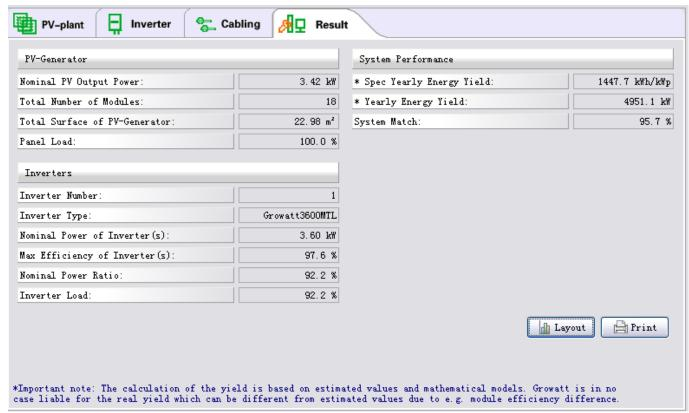
• **Result**: Show the design result information of the PV project includes PV generator, inverters and system match. The Print button at the right corner enables to print the result into PDF documents. And The Layout button enables to set layout of the output PDF documents.
