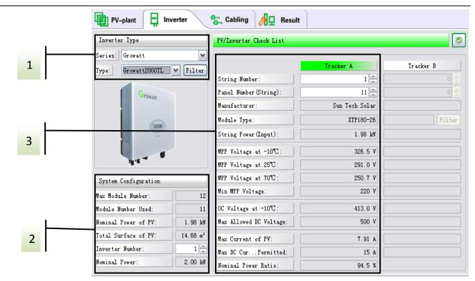
**Filter of Inverters**: Filter the inverters via choose the country or properties of the inverters, or input he inverters series of type (model) to relative boxes.
