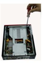
3. Remove the screws from the ODD/HDD bracket with a screwdriver.
