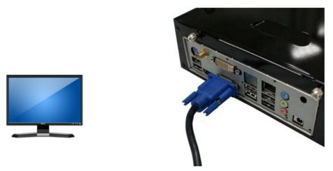
VGA Connector: VGA connector is the 15-pin D-sub female connector; it is for the display devices, such as the CRT monitor, LCD monitor and so on.
