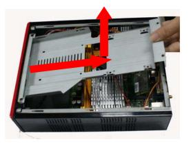
4. Get the bracket out of the chassis before installing memory modules and other devices to the board inside.
