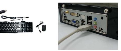
USB Connector: There are 6 USB connectors on rear IO panel to connect USB mouse, keyboard and other USB storage device to the system.
