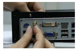
Then lock it to the rear panel with a hexagonal bolt.
