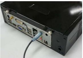
Line-In / Optical SPDIF out shared Connector: This is a line-in connector for user to connect external audio device or to connect Realtek 6-Channel HD Audio CODEC w/ SPDIF out audio output device for superior audio enjoyment.
