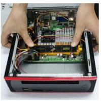
1. Unlock the slot by pushing outwards the eject tabs and then push the module in the right direction downwards vertically.
