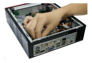
4. Push the other end with screw thread of the 5. antenna string through the antenna hole of the rear panel.
