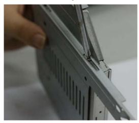
1. Install the optical drive disk to the appropriate position and then lock the screws with a screwdriver.
