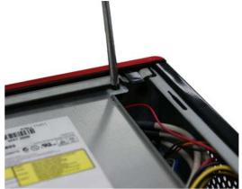
5. Lock the ODD/HDD bracket to the chassis by locking the screws with a screwdriver.
