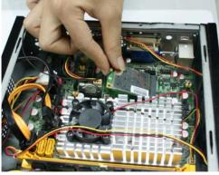
2. Insert the gold figure side of the compatible Mini-PCI-E card into the Mini-PCI-E slot by 45 angle.
