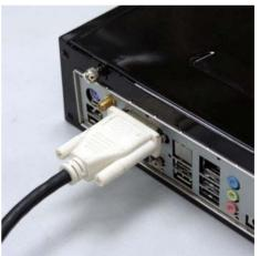
DVI (Digital Visual Interface) Connector: This interface standard designed to maximize the visual quality of digital display devices such as flat panel LCD computer displays and digital projectors.
