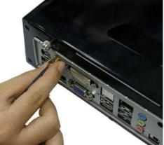
Lock the two big screws on the rear panel to its original place until it firmly locked.
