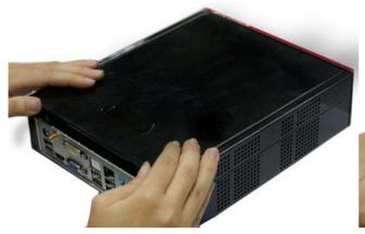
1. Slide the top cover into the chassis and put it 2. in the direction towards the front panel to make sure it firmly locked.
