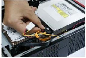
6. Connect the ODD power cable to the ODD. 7.
