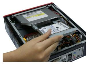
4. Pull the bracket with ODD and HDD locked with screws on it into the ODD/HDD bay.
