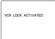
**To turn on,** hold down REC on the DECK in Stop mode with no tape inserted for 7 sec. (Please ignore the NO CASSETTE warning.)
