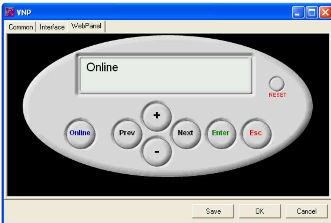
The WebPanel can be used in exceptional cases to set up printer emulations. If you are using a printer that has no GUI print driver the WebPanel allows you to change the printer settings. When using windows print drivers the WebPanel is not required.
