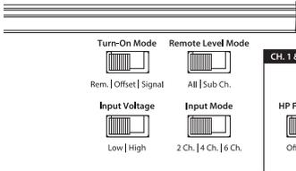
If you wish to send six discrete channels into the XD700/5v2, simply use all six inputs and set the “**Input Mode**” switch in the “**6 Ch.**” position. The amplifier will automatically combine the left and right “**Sub Ch.**” input signals to mono. If you have only one channel of subwoofer signal available, it is acceptable to only use one of the “**Sub Ch.**” inputs, but for optimal gain, we recommend using a Y-adaptor and feeding both “**Sub Ch.**” inputs.
