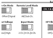
**“Remote Level Mode” Switch:** This switch allows you to assign the operation of the HD-RLC to the entire amplifier or only the subwoofer channel. In the “All” position, the HD-RLC knob will affect all channels equally. In the “Sub Ch.” position, only the level of the subwoofer channel will be affected by the HD-RLC knob.
