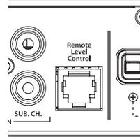
With the addition of the optional Remote Level Control (HD-RLC), you can control the volume of the subwoofer channel (Subwoofer Level) or of the entire XD700/5v2 from the front of the vehicle (Master Volume).
