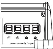
You will notice that there are two “+” positive connections and two “-” negative connections. This is to facilitate multiple subwoofer wiring.
