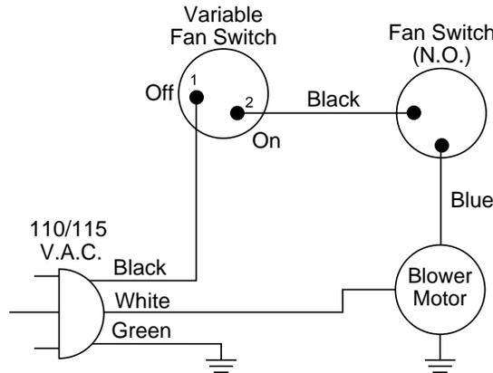
*Figure 61 - Blower Wiring Diagram for Thermostat-Controlled Models*
