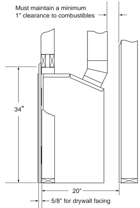
Figure 5 - Framing Clearances for Typical Fireplace Installation
