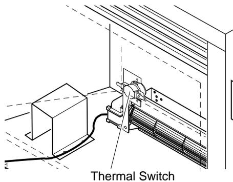
Figure 30 - Locating Thermal Switch Against Back of Firebox
