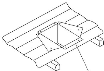
Non-hardening Mastic under all edges of support box before nailing
