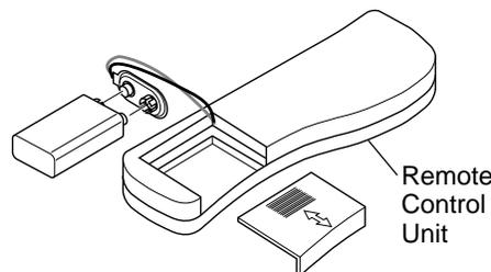
**Figure 43 - Installing Battery in Hand-Held Remote Control Unit (GHRCTA Series Only)**
