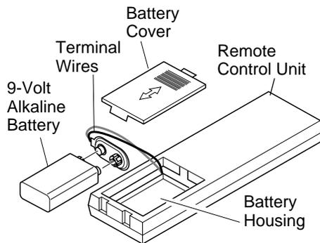
**Figure 42 - Installing Alkaline Battery in Hand-Held Remote Control Unit**
