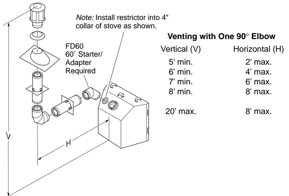
**Figure 25 - Vertical Rigid Venting Configuration Using One 90° Elbow**
