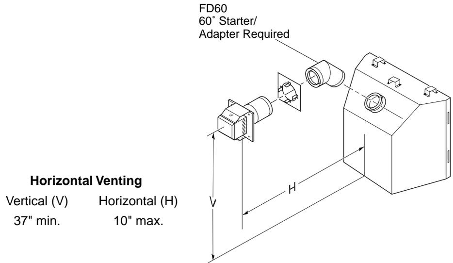
**Figure 16 - Horizontal Termination Configuration for Rigid Venting**
