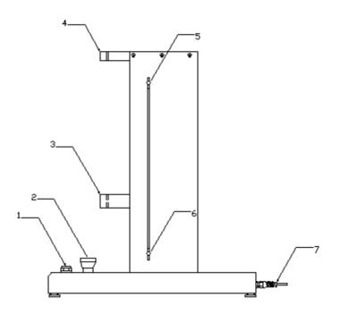
1 – On/off button: must be pressed to turn on the machine. When pressed a lamp inside the button will light, indicating the machine is ready.
