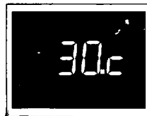
Model has heating function(selecting): Length display Actual temperature, Flashing display set up temperature.
