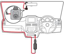
4. When adjusting the angle of mounting, make sure that the camera's view is parallel with the level ground, and the ground/sky ratio is close to 6/4.
