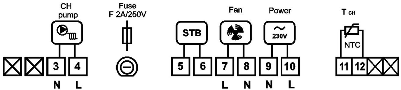
Fig. 1 Diagram of connections between equipment, sensors and the GH09NB controller
