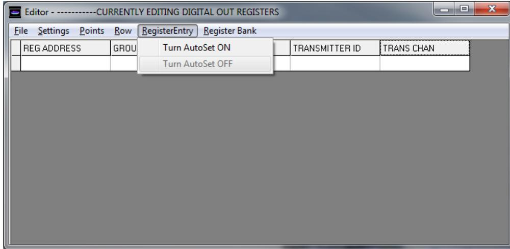
Enter the Register address in the REG ADDRESS window. The valid range is 0 to 49.
