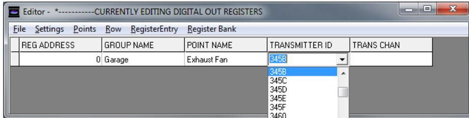
Assign the appropriate digital or relay output “TRANS CHAN” to the data register by clicking in the cell to open a drop down menu. Click on the appropriate transmission channel (01 to 04) to select.
