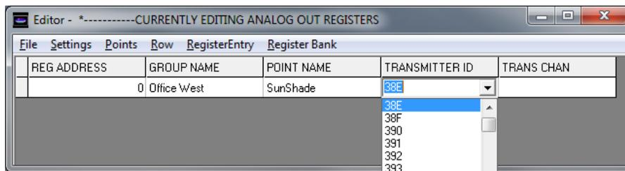
Assign the appropriate digital or relay output “TRANS CHAN” to the data register by clicking in the cell to open a drop down menu. Click on the appropriate transmission channel (01 to 04) to select.
