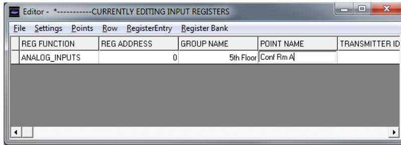
Assign a sensor/transmitter to the data register by clicking in the TRANSMITTER ID cell to open a drop down menu. Use the scroll bar to scroll to the correct address or automatically scroll to the address by typing the hexadecimal address in the cell. To select the address click on the appropriate ID in the drop down menu. Each ACI wireless transmitter is factory configured with a unique ID – refer to the sensor product data sheet for the location of the transmitter ID.
