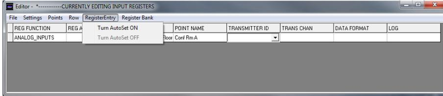
Enter the Register address in the REG ADDRESS window and press down arrow to enter.
