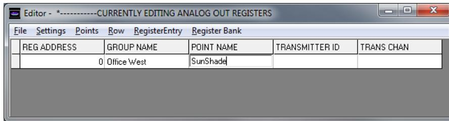
Assign a sensor/transmitter to the data register by clicking in the TRANSMITTER ID cell to open a drop down menu. This is the device ID of the remote output devices (RD2432). Use the scroll bar to scroll to the correct address or automatically scroll to the address by typing the hexadecimal address in the cell. To select the address click on the appropriate ID in the drop down menu.
