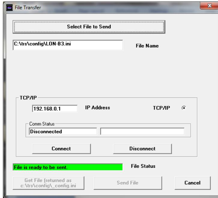
Click on “Connect” and the status of the connection will be displayed in the Comm Status window. When the Transceiver is connected click on “Send File” to the send the config file to the Transceiver.
