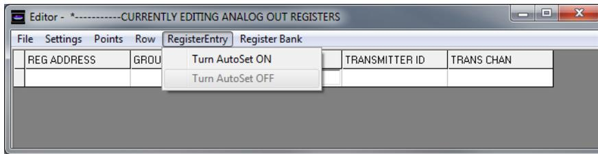
Enter the Register address in the REG ADDRESS window. The valid range is 0 to 49.
