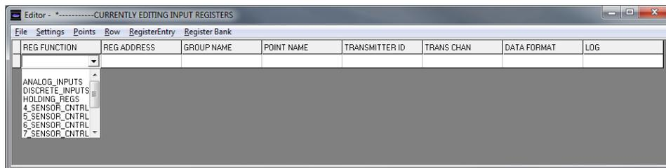
Use the mouse to move to the next column to assign the REG ADDRESS by clicking in the cell. Before entering register addresses, ensure the “RegisterEntry” AutoSet is turned off as shown:
