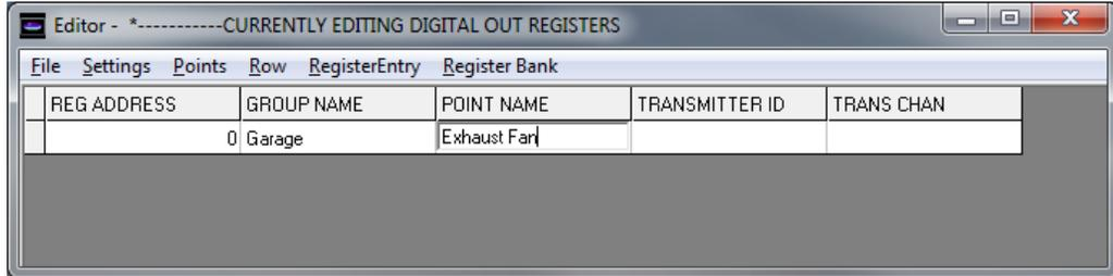
Assign a sensor/transmitter to the data register by clicking in the TRANSMITTER ID cell to open a drop down menu. This is the device ID of the remote output devices (RD2402 & RD2432). Use the scroll bar to scroll to the correct address, or automatically scroll to the address by typing the hexadecimal address in the cell. To select the address click on the appropriate ID in the drop down menu.
