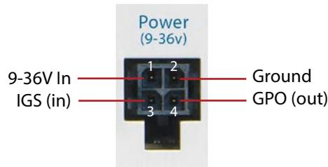
Figure 5: Power Connector Pin Assignments
