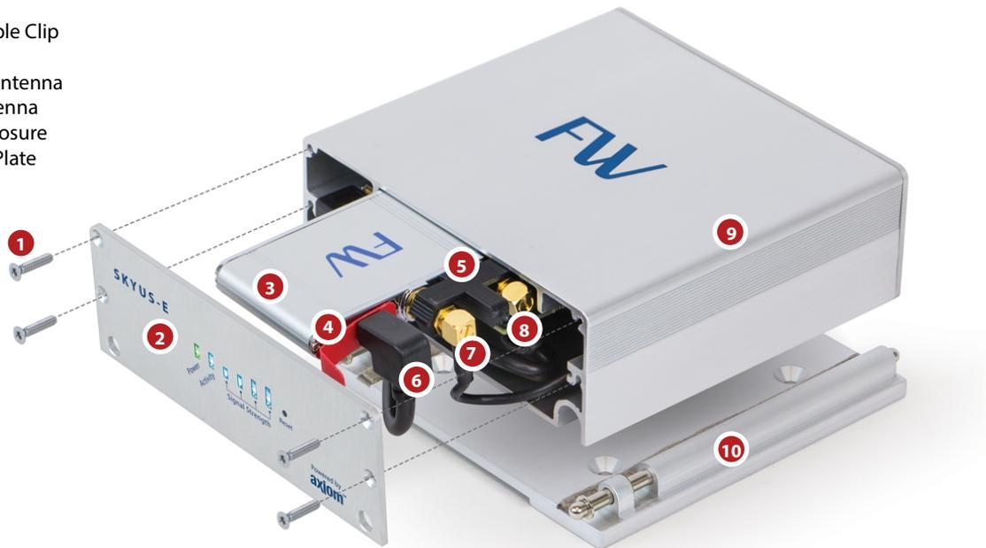
Figure 7: Skyus Modem Installation (Single SIM Modem)
