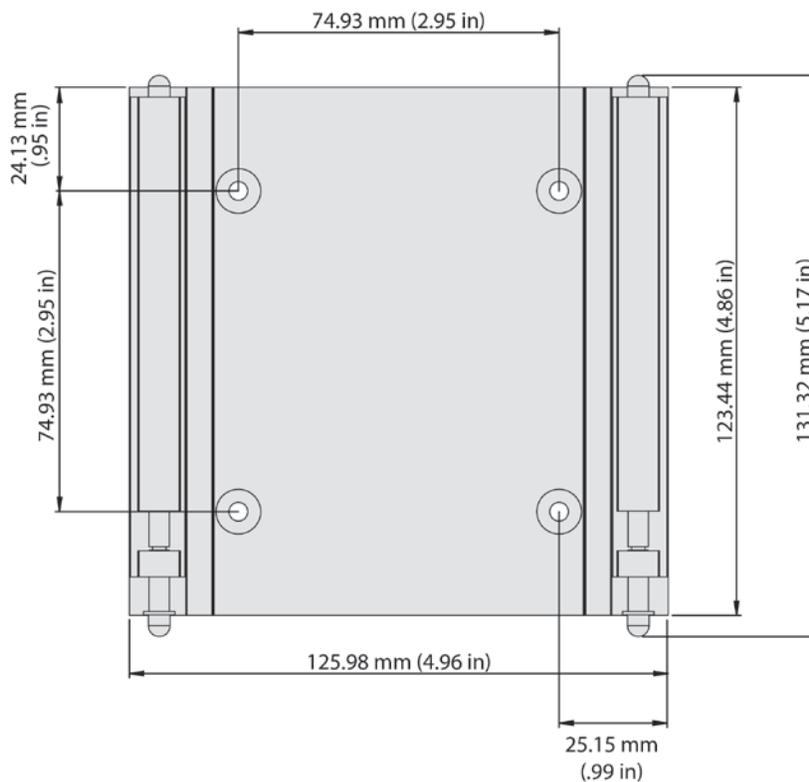
Figure 2: Mounting Plate Dimensions (Not to scale.)
