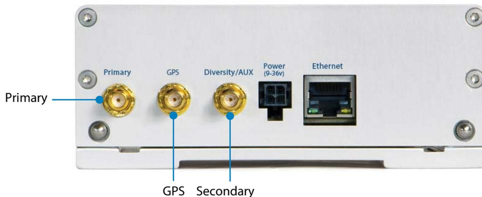
Figure 4: Antenna Connections
