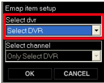
Aside from Camera or Sensor icon display on E-map, separate DVR icon can be positioned on the E-map. The DVR icon will be blinking any event which is happening on the same DVR.
