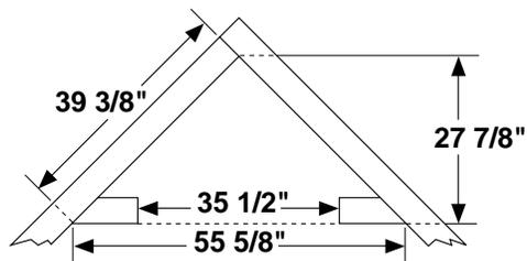
**Figure 13 - Rough Opening for Installing in Corner**
