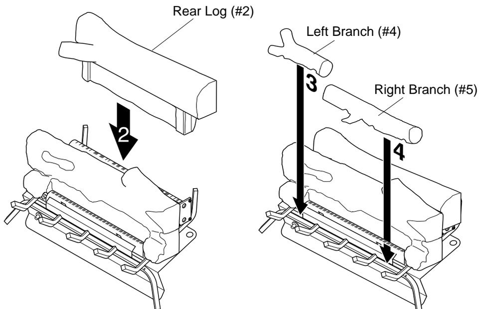
**Figure 23 - Installing Rear Log**
