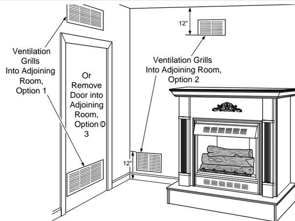
Figure 3 - Ventilation Air from Inside Building
