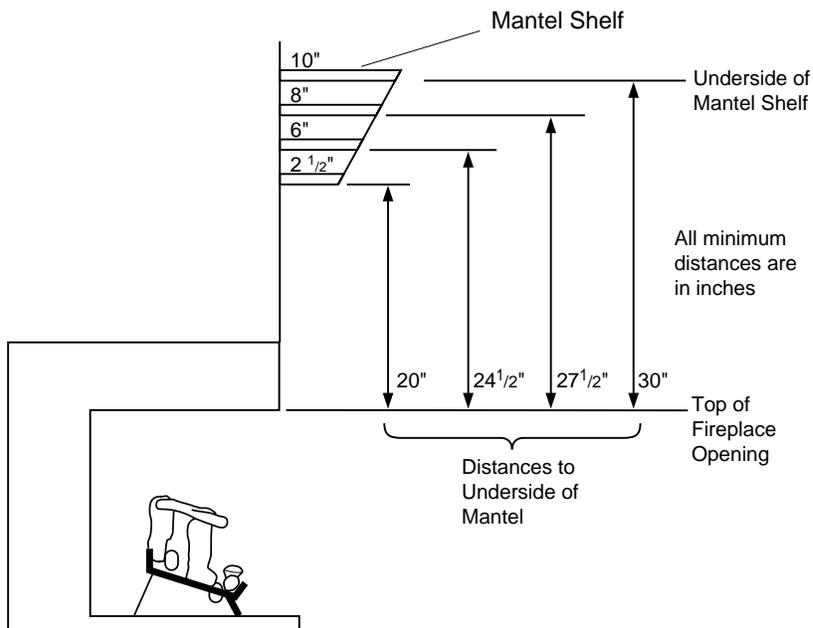
**Figure 15 - Minimum Mantel Clearances for Built-In Installation**
