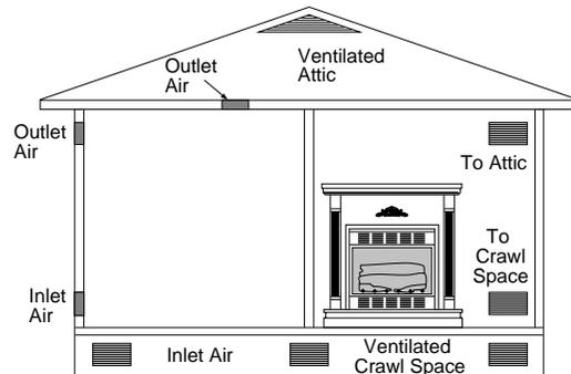
Figure 4 - Ventilation Air from Outdoors
