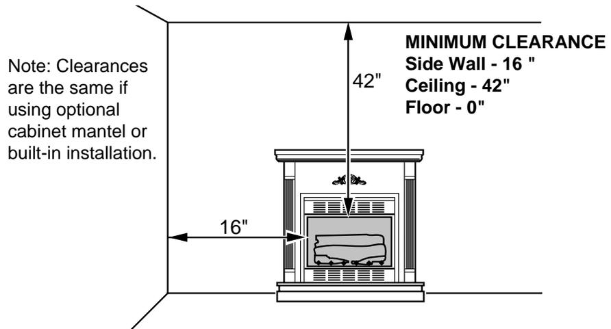
*Figure 7 - Minimum Clearance to Wall and Ceiling*
