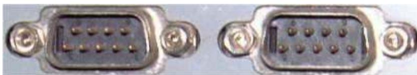
Figure 3 – PC serial communication ports
