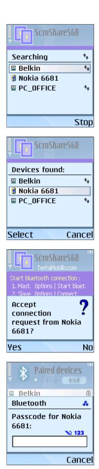
Wait until the right device has been found. You can <u>stop</u> <u>the bluetooth search process</u> by pressing the right selection key (Stop) as soon as your device has been found. This avoids having to wait until all bluetooth devices have been found which potentially can take a long time.
