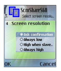
screen images are to be sent in their original high resolution format (352 x 416). Images are automatically scaled down to 176 x 208 size when the slave phone is a low resolution phone (no confirmation is asked). This is the <u>default setting</u> when installing ScreenShareS60 and offers a compromise between image quality, sending speed and user control.
