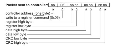
Example (988 only): Set register 7 (SPI) to 200 (0x00C8) on controller at address 9.
