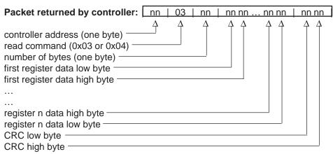
Example (988 only): Read register 0 (model number) of the controller at address 1.
