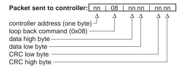
Example: Run loop back test on controller at address 40 (0x28).
