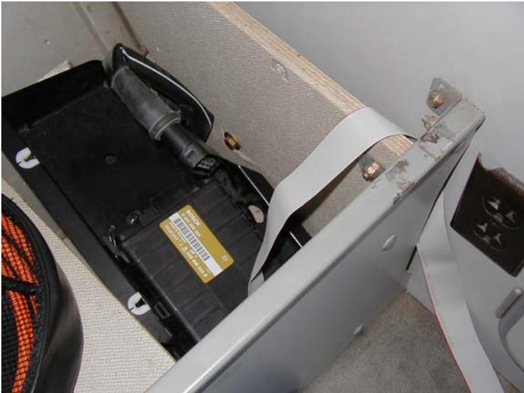
Make sure the gray ribbon cable is positioned as shown, and NOT across the forward rear seat support. Also ensure that the cable you disconnected from your ECU is positioned as shown, on top of the black box, and near the ECU.
