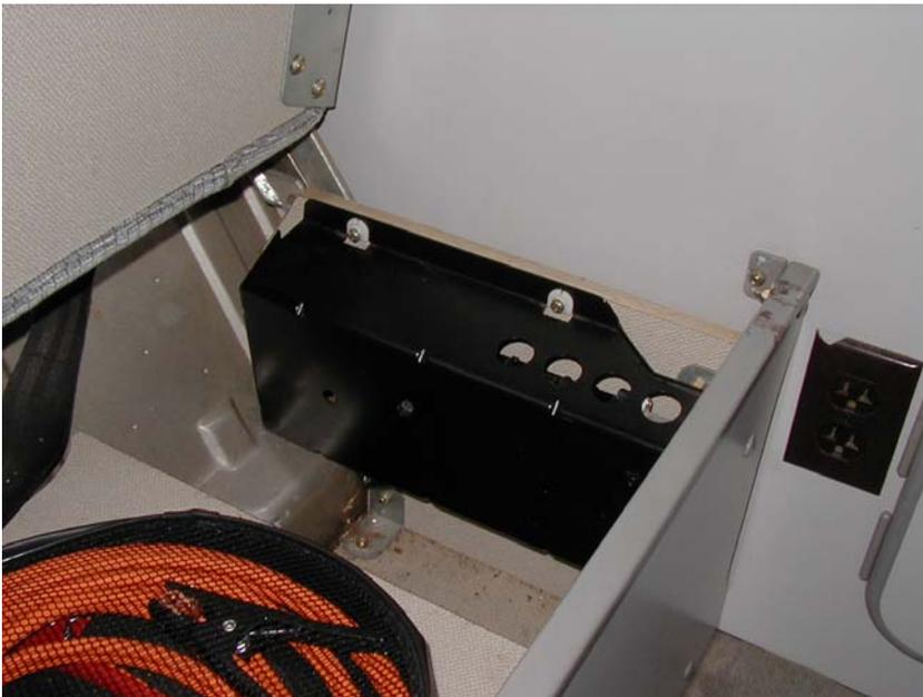
The ECU is inside the rectangular black enclosure. It is held in place with three Phillips head screws, two of which are seen in this photo at the top edge of the black box. The third screw is not visible here, but is located nearly directly below the right hand top screw on the bottom flange of the ECU black box. Loosen, but DO NOT REMOVE the lower screw, and REMOVE the two top screws to unfasten the ECU holder from the right hand seat frame.
