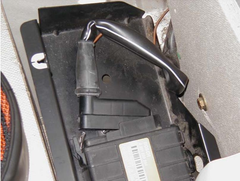
Now remount the ECU assembly back onto the right hand rear seat support. First, position the lower screw slot on the screw even with the bottom of the ECU black box. Once this is done, replace the two upper screws, making them snug, but NOT tight. Route the gray ribbon cable as shown, and lower the rear seat. Your test ECU is installed.
