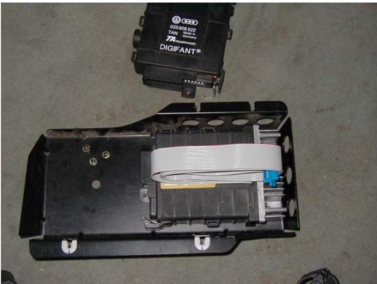
Now place the mounted ECU into the rear seat compartment, laying the black box, open side up, flat in the same position you removed your ECU a few moments ago. Route the ribbon cable ABOVE the right seat frame, and THROUGH the narrow opening in the rear seat vertical support as shown:
