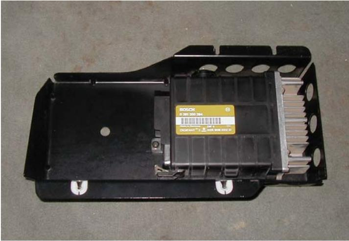
You will now need to remove the ECU from its black box holder, by removing the three Phillips head screws that fasten it to the black box. Each of these has a flat washer and a lock washer. I usually let the hardware fall into the black box, as the test ECU will need the same screws.
