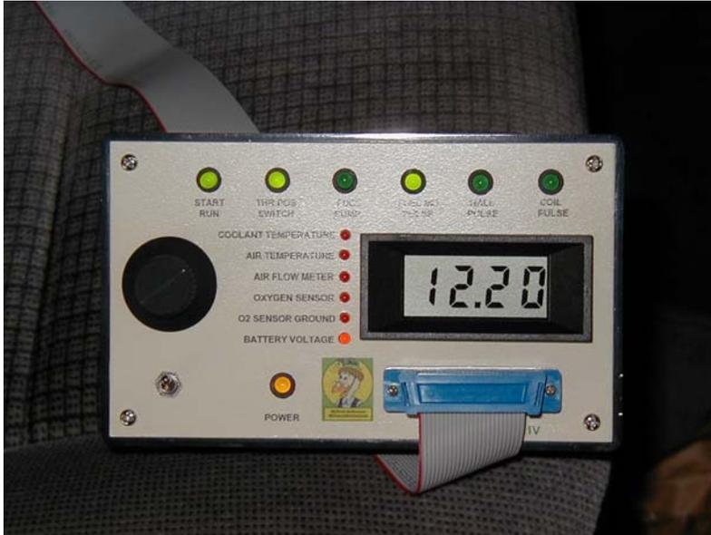
The green START/RUN, THROTTLE POSITION SWITCH, AND INJECTOR PULSE LEDs and the red BATTERY VOLTAGE LED should illuminate. The digital display should display approximately 12V.
