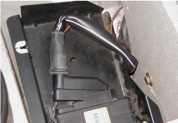
Now remove the electrical connector by swinging it up and to the right, removing the small tab from the opening at the right end of the connector socket.
