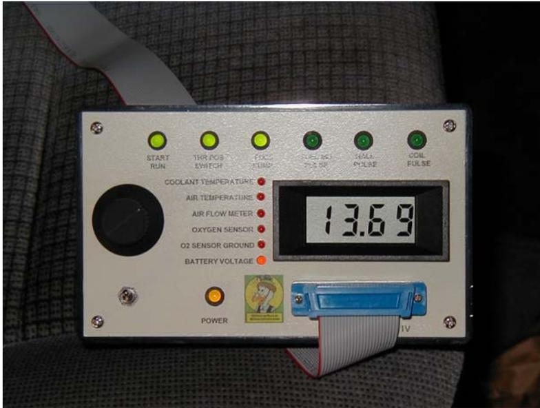
Now rotate the selector switch to the full counterclockwise position, COOLANT TEMPERATURE. This should illuminate the red coolant temperature indicator, and the digital display should indicate approximately .95 V. This value will depend on the coolant temperature at the time.
