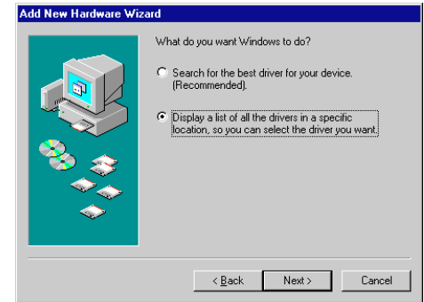
Figure 7: Selecting the option Display a list of all the drivers in a specific location, so you can select the driver you want.
