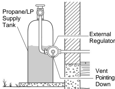
**Figure 19 - External Regulator with Vent Pointing Down**
