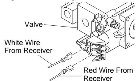
**Figure 29 - Connecting Wires**
