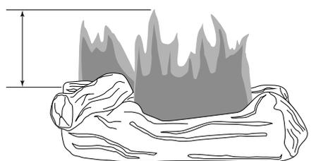
Figure 40 - Incorrect Flame Pattern with Control Knob Set to High Flame
