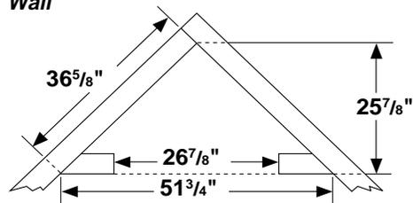
Figure 6 - Rough Opening for Installing in Corner
