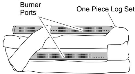
**Figure 26 - Installing One-Piece Log set (Top View)**
