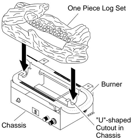
**Figure 25 - Installing One-Piece Log Set**
