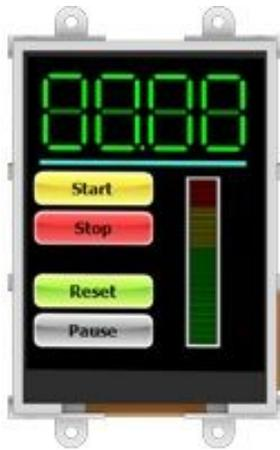
For the needs of the AMRobot platform it is possible to use any display available, however it is recommended to use an intelligent graphic display by *4D Systems* that can be quickly configured by external master microcontroller (*Arduino* for instance) through serial interface (UART). It can also work as a standalone device. The choice of work mode is accomplished by a public configuration file available on *4D Systems* website.
