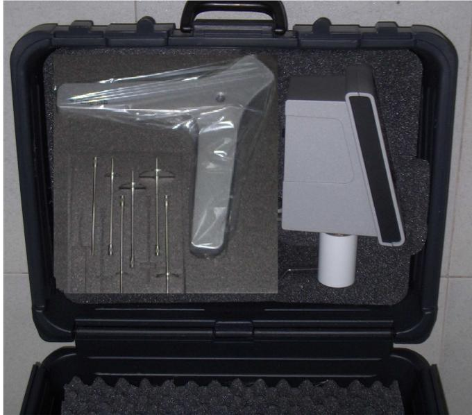
Fig 1. The viscometer in its carry-case
