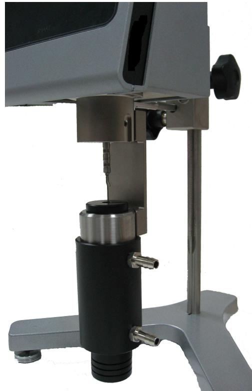
Fig.9: LCP Adapter assembled in viscometer
