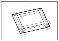
**5.** Release the locking system to remove the internal glass panel.
