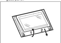
8. Clean the glass panel with water and soap. Dry the glass panel carefully. When the cleaning is completed, install the glass panel and the oven door. Do the above steps in the opposite sequence.
