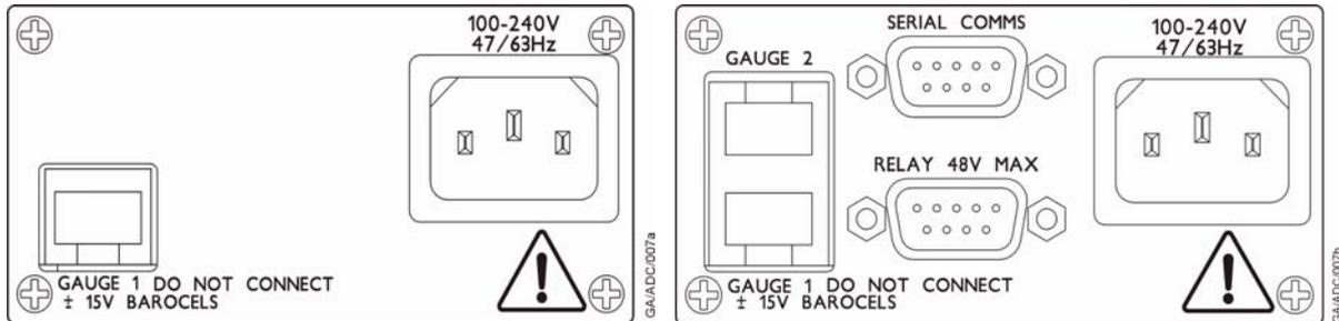
Figure 7 - Rear panel connections
