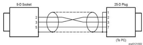
Figure 9 - IBM PC RS232 interface - 25-way
