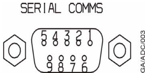
Figure 3 - Pin connections for the serial comms connector
