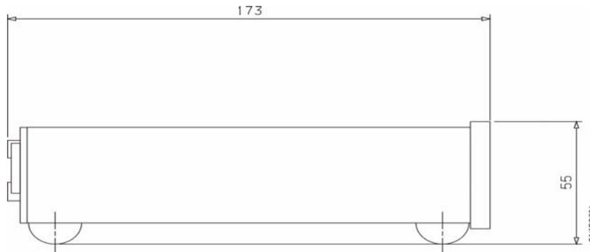
Figure 4 - Bench mounted dimensions (mm)
