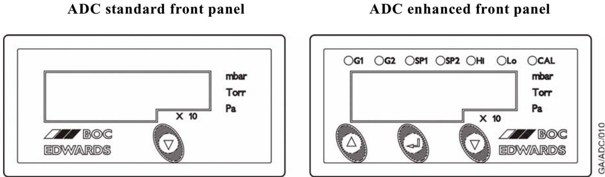
Figure 10 - Front panel displays
