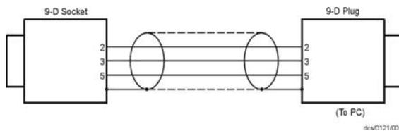
Figure 8 - IBM PC RS232 interface - 9-way
