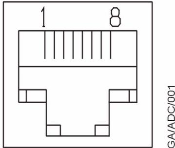
Figure 1 - Pin connections for an 8-way FCC/RJ45
