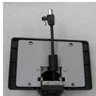
5. Install USB cable to monitor screws
