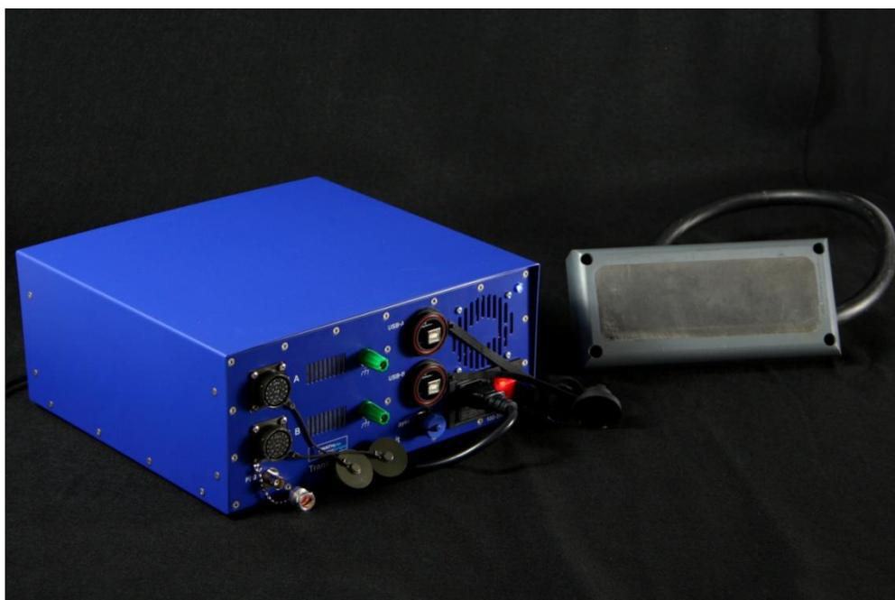
**Figure 3-1** The Bathyswath base system comprises a Transducer Interface Unit (left shows one type- others are available) and two sonar transducers (Bathyswath-H shown right).
