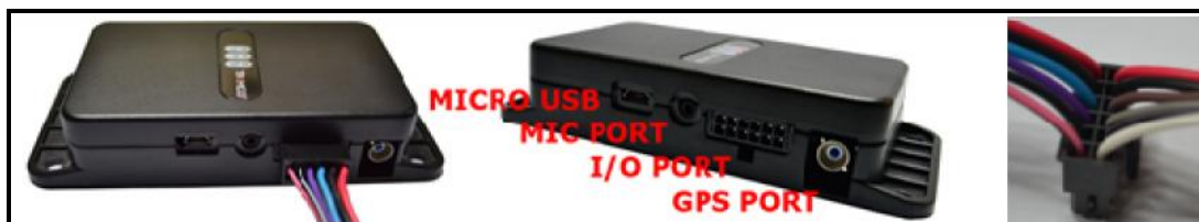
Figure 3 - T23 and T23 Fleet I/O port & I/O cable
