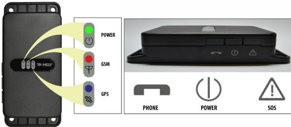
Figure 6 - T23 and T23 Fleet lights and buttons
