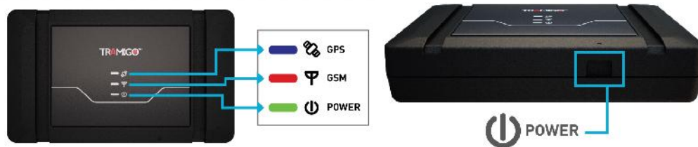
Figure 7 - T23 Track lights and button
