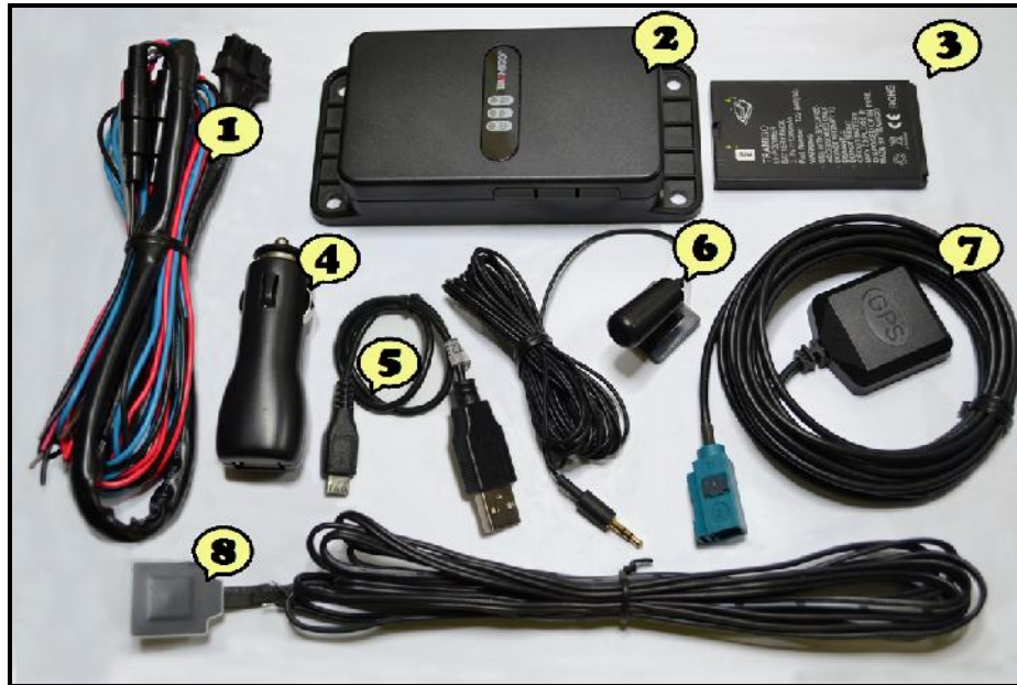
Figure 1 – T23 and T23 Fleet and Automotive Installation Kit
