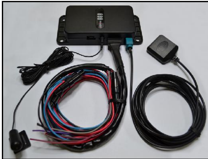
Figure 8 – T23 and T23 Fleet automotive installation/Wires connected
